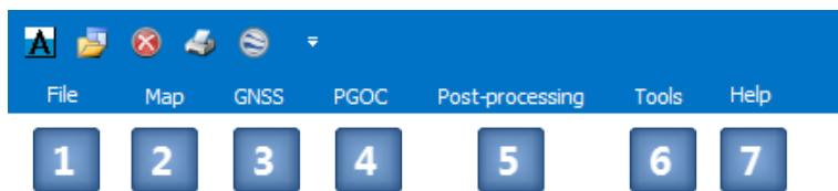
The **Manage** toolbar is the main toolbar of *ArpentGIS-Expert* software and allow the user to navigate within the **map** view, access to the measurement functions or launch the various software wizards (post-processing, Data dictionary editor, File Transfer, Registration of the software, Options...)
